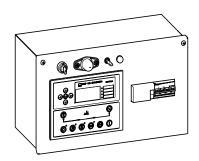
PLC-7420 is an advanced control module based on microprocessor, containing all necessary functions for protection of the genset and the breaker control. It can monitor the mains supply, and automatically start the engine when the mains is abnormal. Accurately measure various operational parameters and display all values and alarms information on the LCD. In addition, the control module can automatically shut down the engine and indicate the engine failure.
